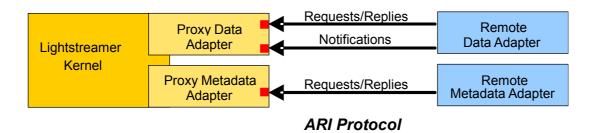
The Proxy Data Adapter and the Proxy Metadata Adapter are ready-made Adapters, written in Java and provided as part of the ARI SDK. They run in-process with Lightstreamer Server and expose the Data Provider and Metadata Provider interfaces over TCP/IP sockets.
